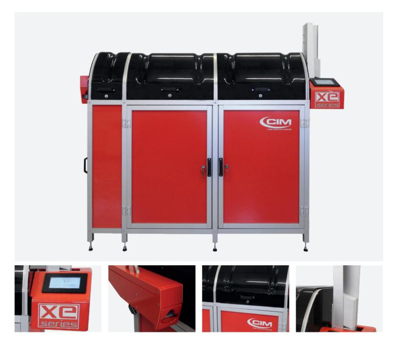
The new XE SERIES design is based on combination of two or more basic elements (BIG and SMALL) in order to provide a cabinet for any more or less complex composition of personalization Modules. The modular structure is characterized by electronic components produced for industrial market, so that they are robust and being easily integrated.
